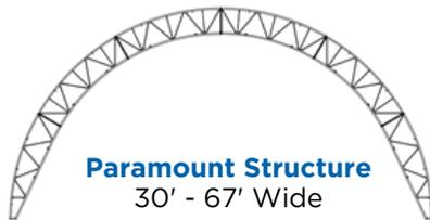
The Paramount building series was developed as a heavy snow load, trussed solution for the agriculture and heavy industrial sectors. Our High Profile Paramount utilizes a straight leg frame, which can maximize square footage and allow for side entry doors.
